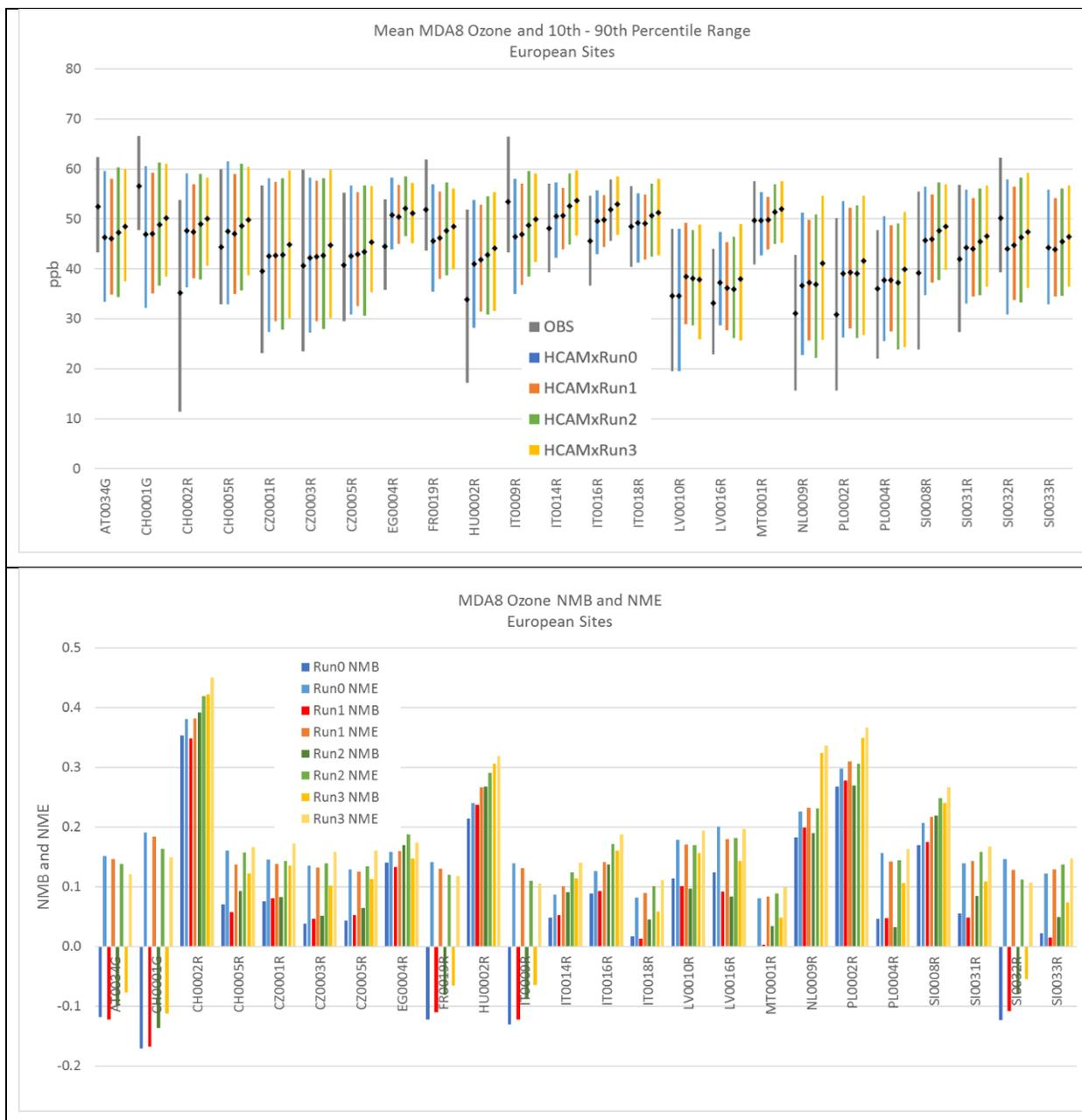
**Figure 4-18. Measured and H-CAMx annual average (black dots) and 10<sup>th</sup>-90<sup>th</sup> percentile ranges (vertical bars) of surface ozone by European site (top panel), and modeled statistical performance metrics for bias (NMB as decimal fraction) and gross error (NME as decimal fraction) by European site (bottom panel). Observations are shown in grey, H-CAMx results are shown in color.**
