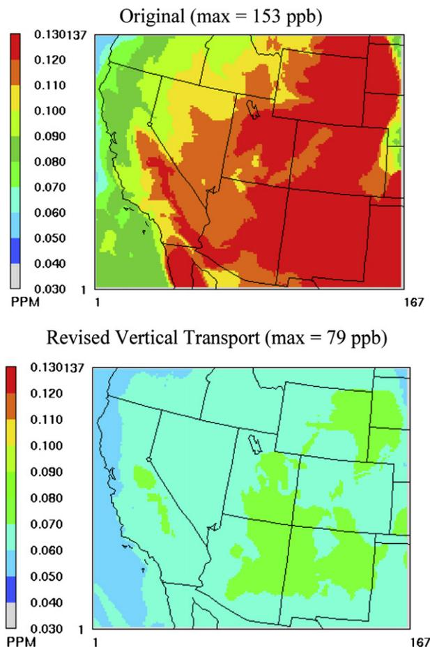
Fig. 5. April 2005 CAMx inert maximum ozone concentrations (ppm) using “zero-gradient” top BC, 2005 lateral BC, and original 19 layer vertical structure; original model (top) and revised vertical advection algorithm (bottom).
