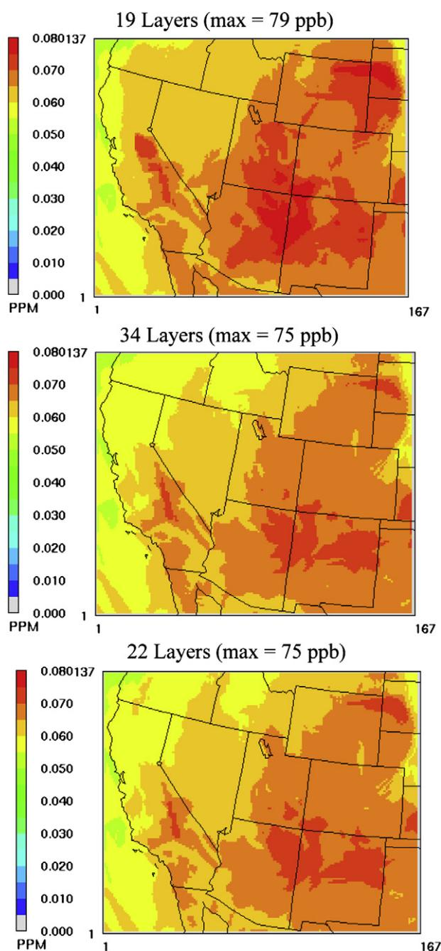
**Fig. 6.** April 2005 CAMx inert maximum ozone concentrations (ppm) using “zero-gradient” top BC, 2005 lateral BC, and revised vertical advection algorithm; original 19 layer vertical structure (top), 34 layer structure (middle), and 22 layer structure (bottom).
