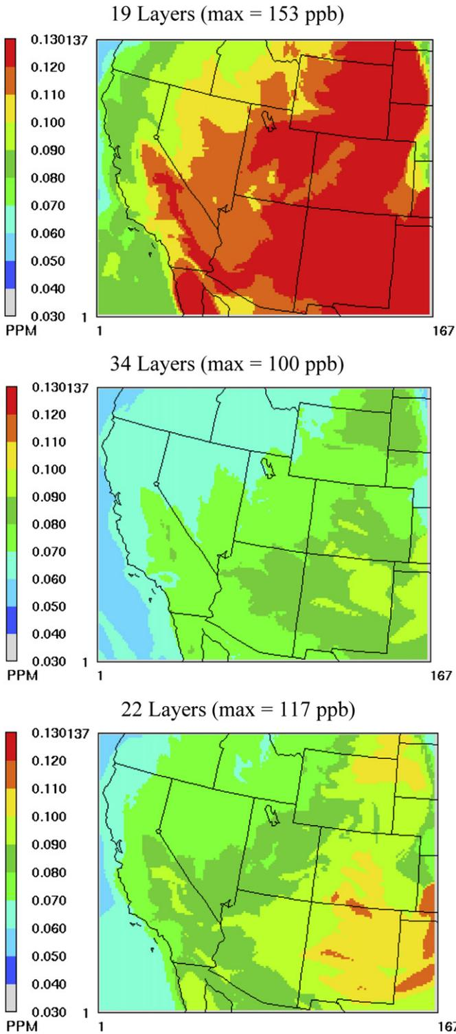
Fig. 3. April 2005 CAMx inert maximum ozone concentrations (ppm) using “zero-gradient” top BC, 2005 lateral BC, and original 19 layer vertical structure (top), full 34 layer vertical structure (middle) and intermediate 22 layer vertical structure (bottom).
