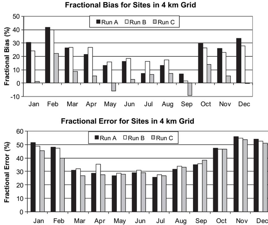
Fig. 9. Monthly ozone fractional bias (top) and error (bottom) for CAMx Runs A, B, and C based on all ozone measurements within the 4-km modeling domain.
