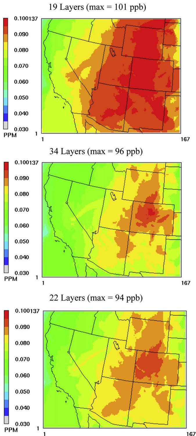
Fig. 2. April 2005 CAMx inert maximum ozone concentrations (ppm) using “zero-gradient” top BC and original 19 layer vertical structure (top), full 34 layer vertical structure (middle) and intermediate 22 layer vertical structure (bottom).
