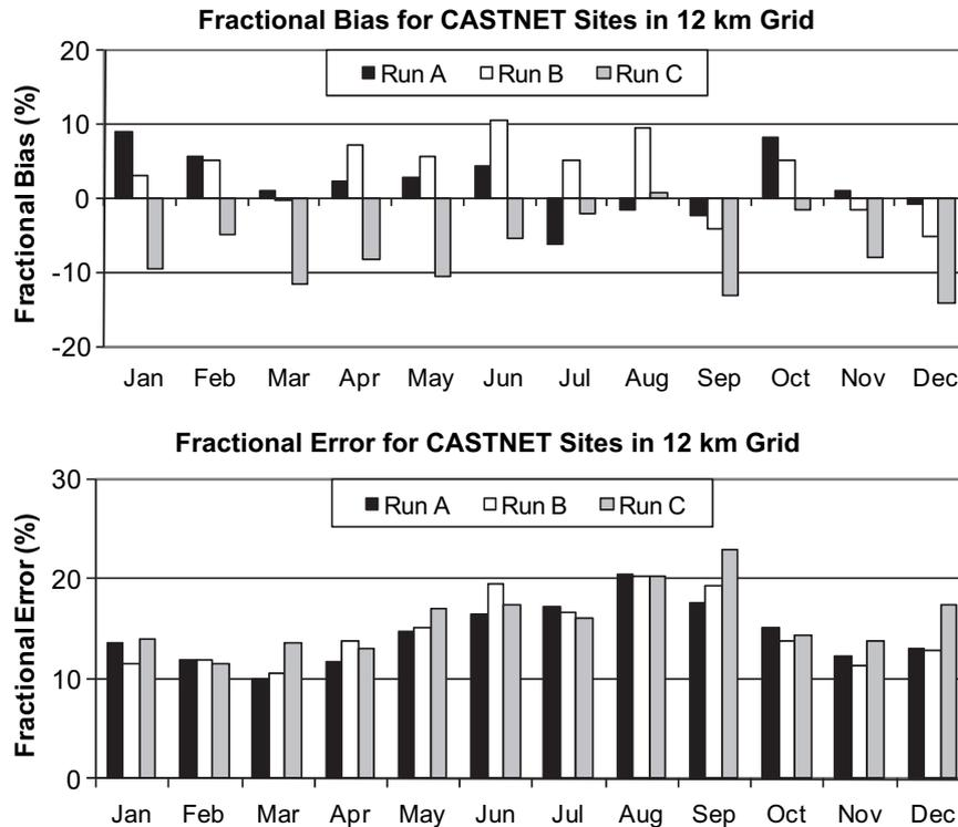
Fig. 10. Monthly ozone fractional bias (top) and error (bottom) for CAMx Runs A, B, and C based on selected high-elevation CASTNET ozone measurements within the 12-km modeling domain.
