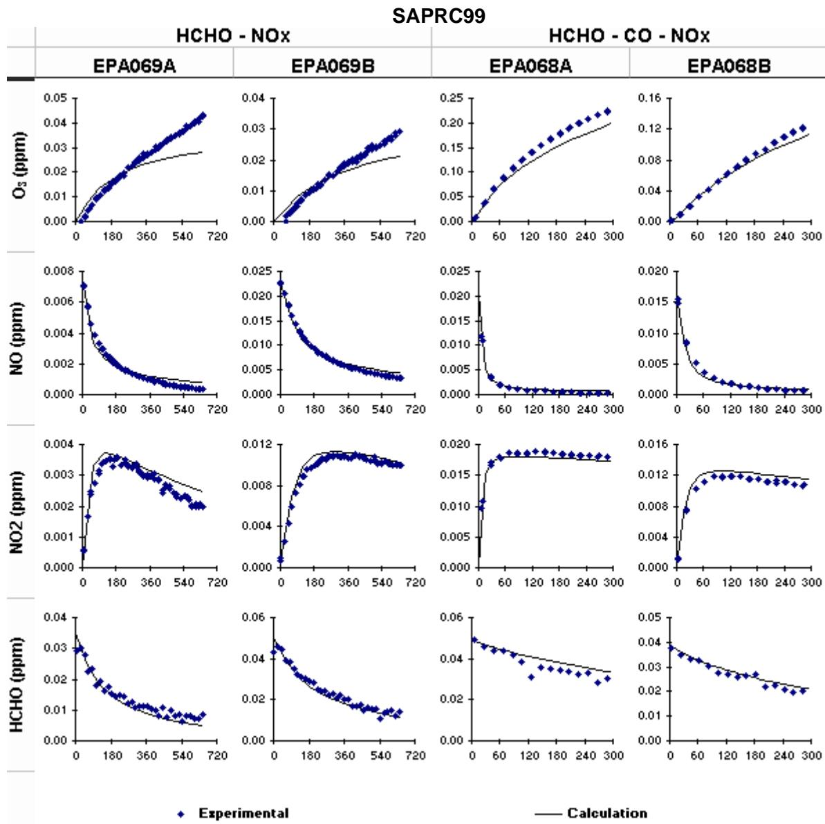
**Figure 4-7.** SAPRC99 simulation of four formaldehyde experiments in the EPA chamber at UCR.
