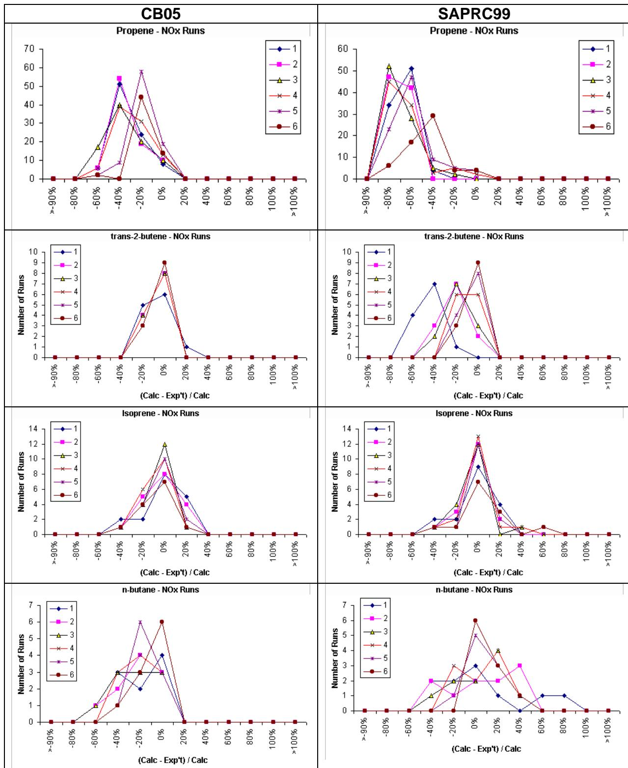
**Figure 4-16. (continued).** Bias in oxidant production ( $O_3$ -NO) at hours 1-6 in UCR chamber experiments for the CB05 and SAPRC99 mechanisms, by compound.
