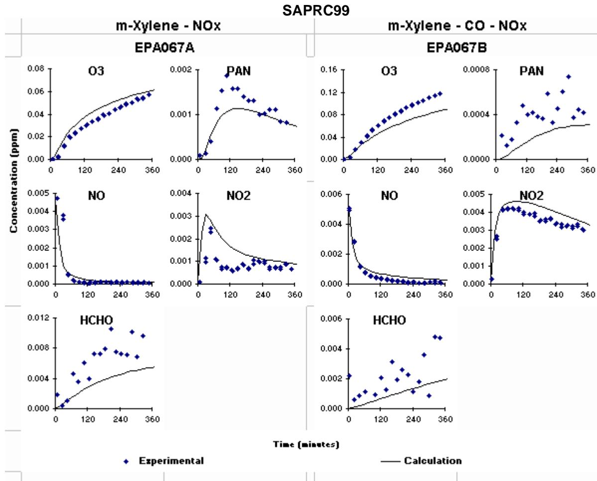
**Figure 4-14.** SAPRC99 simulation of two xylene experiments in the EPA chamber at UCR.
