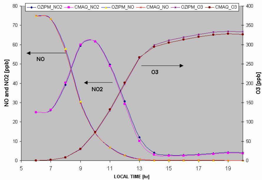
**Figure 3-7.** Comparison of results from the CMAQ and OZIPM box models for NO, NO<sub>2</sub> and O<sub>3</sub> at 298 K and 1 atmosphere.
