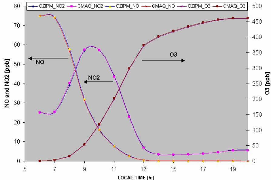
**Figure 3-9.** Comparison of results from the CMAQ and OZIPM box models for NO, NO<sub>2</sub> and O<sub>3</sub> at 298 K and 0.5 atmosphere.
