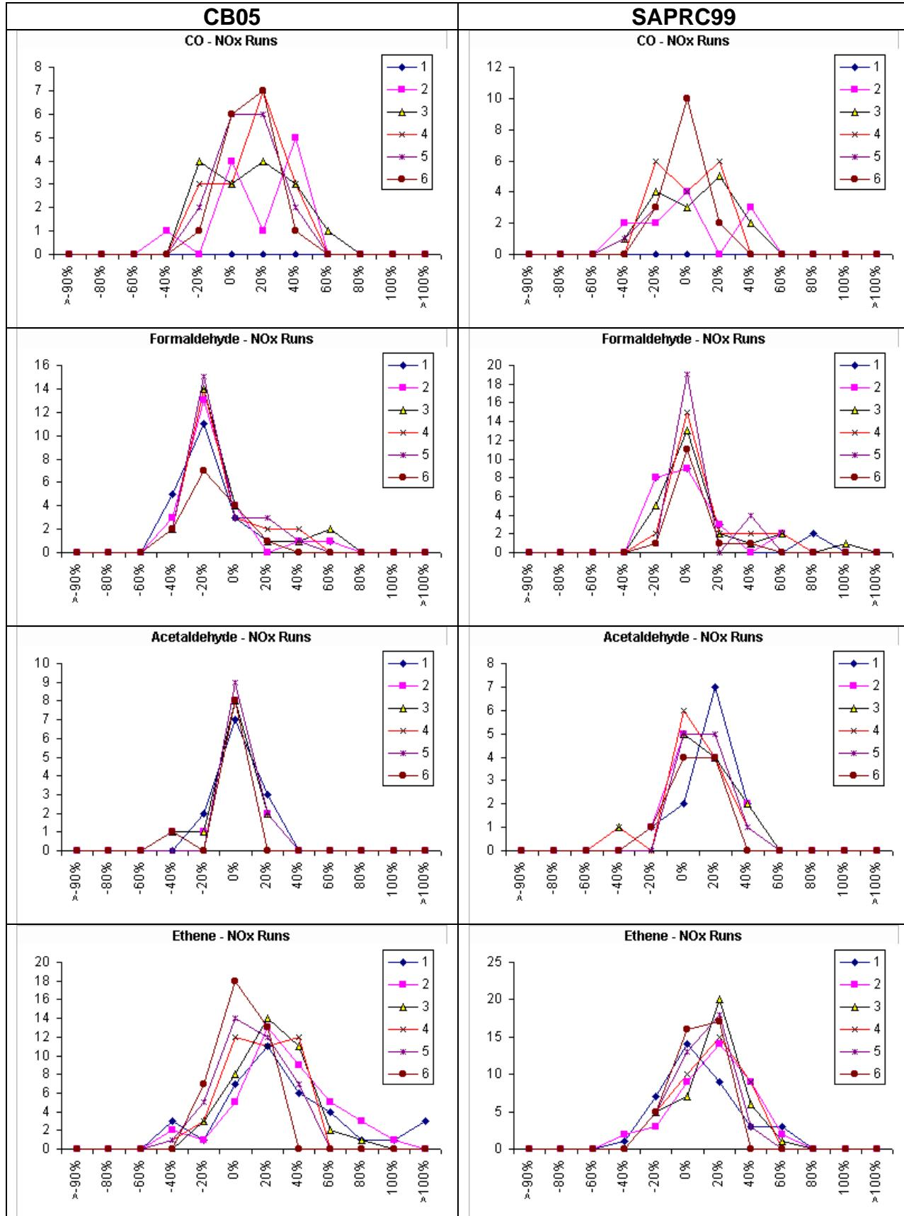
**Figure 4-16.** Bias in oxidant production ( $\text{O}_3\text{-NO}$ ) at hours 1-6 in UCR chamber experiments for the CB05 and SAPRC99 mechanisms, by compound.
