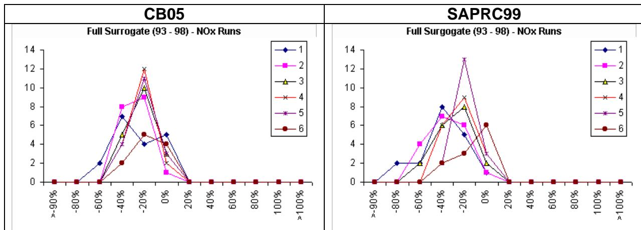
**Figure 4-16.** (concluded). Bias in oxidant production ( $O_3$ -NO) at hours 1-6 in UCR chamber experiments for the CB05 and SAPRC99 mechanisms, by compound.
