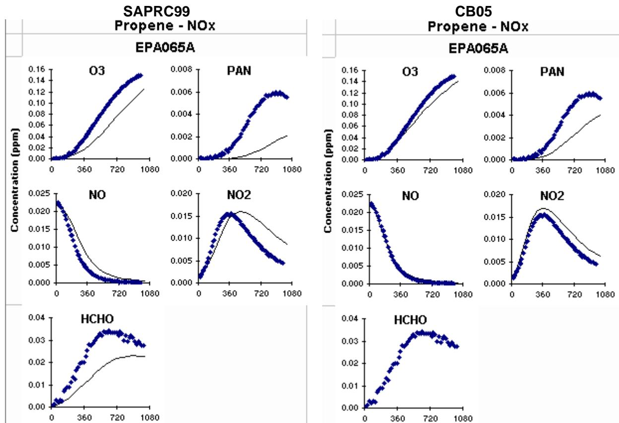
**Figure 4-10.** SAPRC99 (left) and CB05 (right) simulation of a propene experiment in the EPA chamber at UCR.
