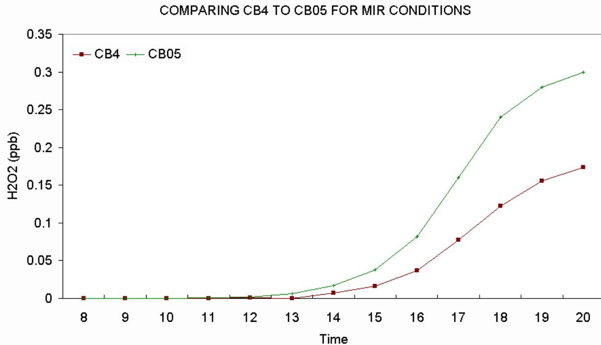
**Figure 3-3.** Comparison of CB4 and CB05  $\text{H}_2\text{O}_2$  predictions for urban MIR conditions.
