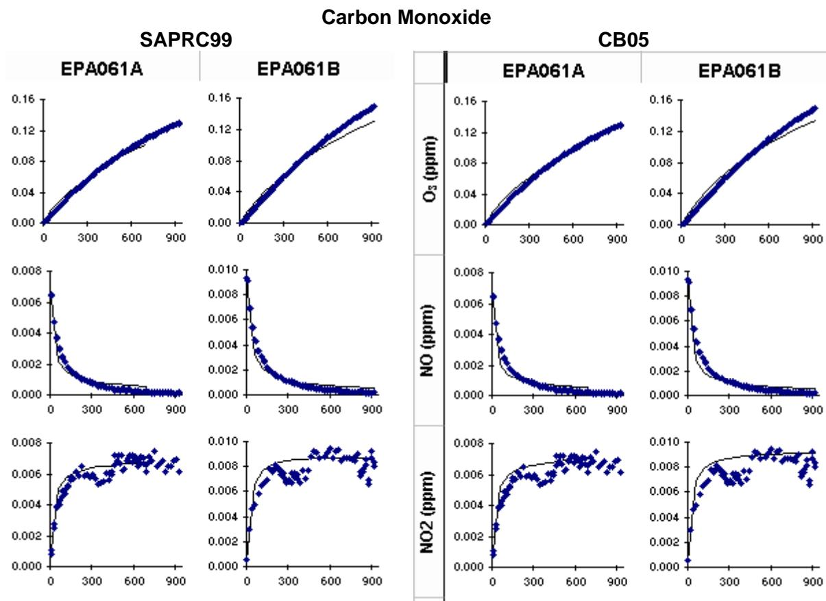
**Figure 4-6.** SAPRC99 (left) and CB05 (right) simulation of a carbon monoxide experiment in the EPA chamber at UCR.
