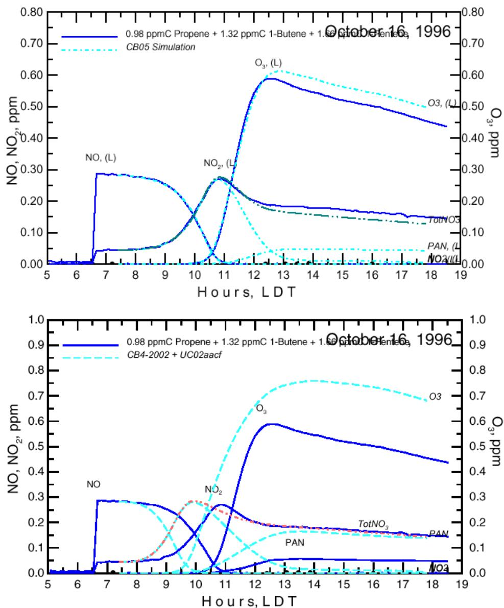
**Figure 4-4.** Comparison of CB05 (top) and CB4-2002 (bottom) simulations of UNC experiment October 16, 1996 (blue chamber) with propene, 1-butene and 1-pentene.
