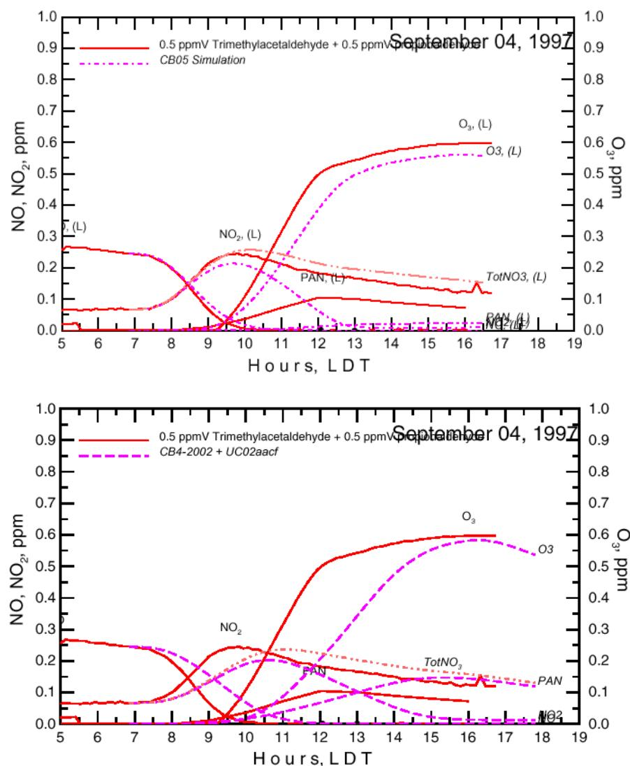
**Figure 4-3.** Comparison of CB05 (top) and CB4-2002 (bottom) simulations of UNC experiment of September 4, 1997 (red chamber) with trimethylacetraldehyde and propionaldehyde.
