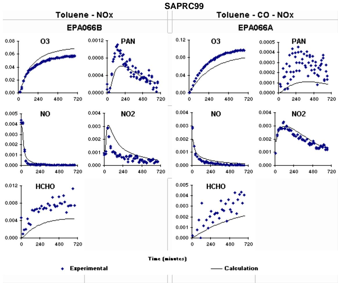
Figure 4-12. SAPRC99 simulation of two toluene experiments in the EPA chamber at UCR.
