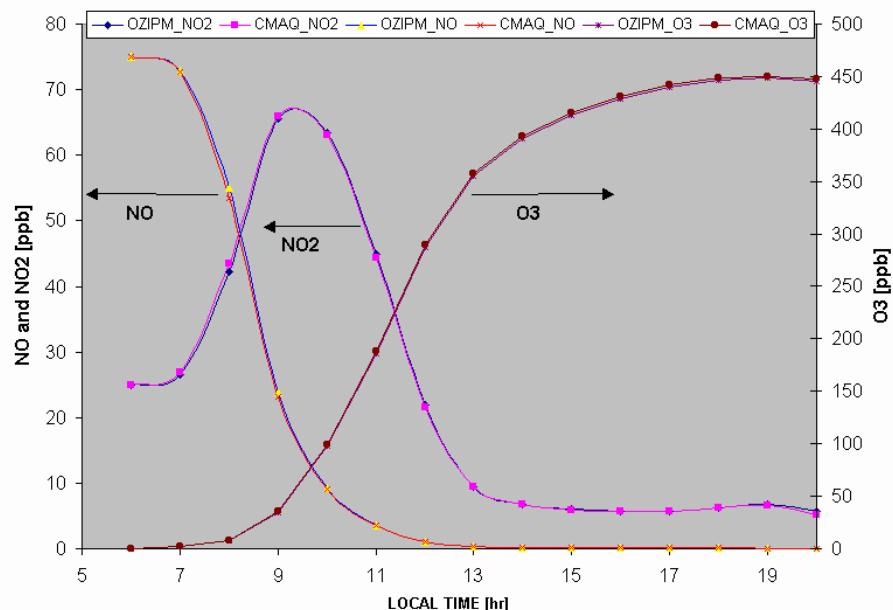
**Figure 3-10.** Comparison of results from the CMAQ and OZIPM box models for NO, NO<sub>2</sub> and O<sub>3</sub> at 310K and 1 atmosphere.
