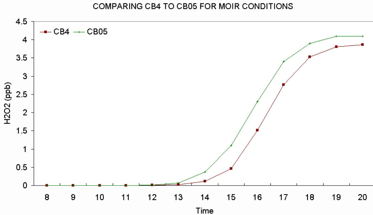
**Figure 3-6.** Comparison of CB4 and CB05  $\text{H}_2\text{O}_2$  predictions for urban MOIR conditions.
