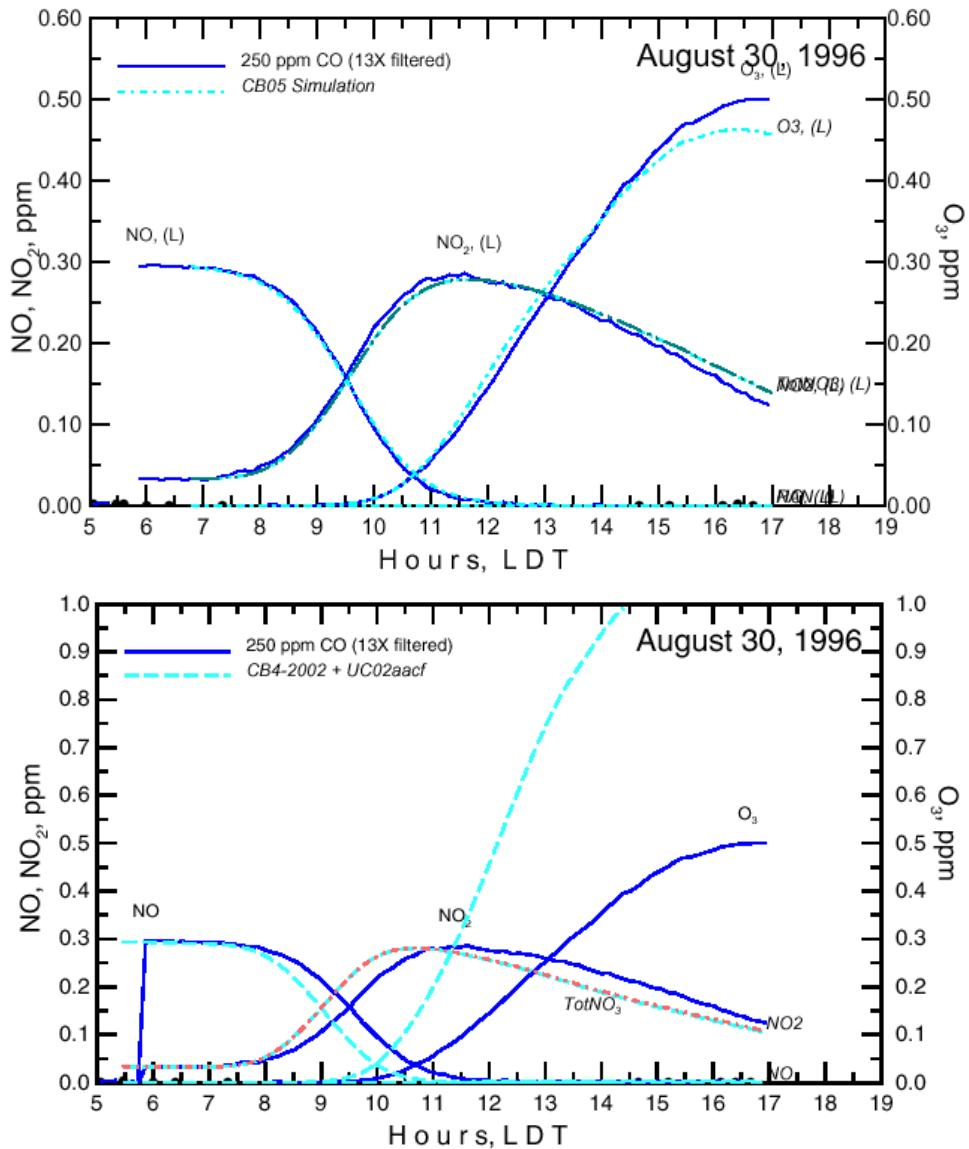
**Figure 4-2.** Comparison of CB05 (top) and CB4-2002 (bottom) simulations of UNC carbon monoxide experiment August 30, 1996 (blue).
