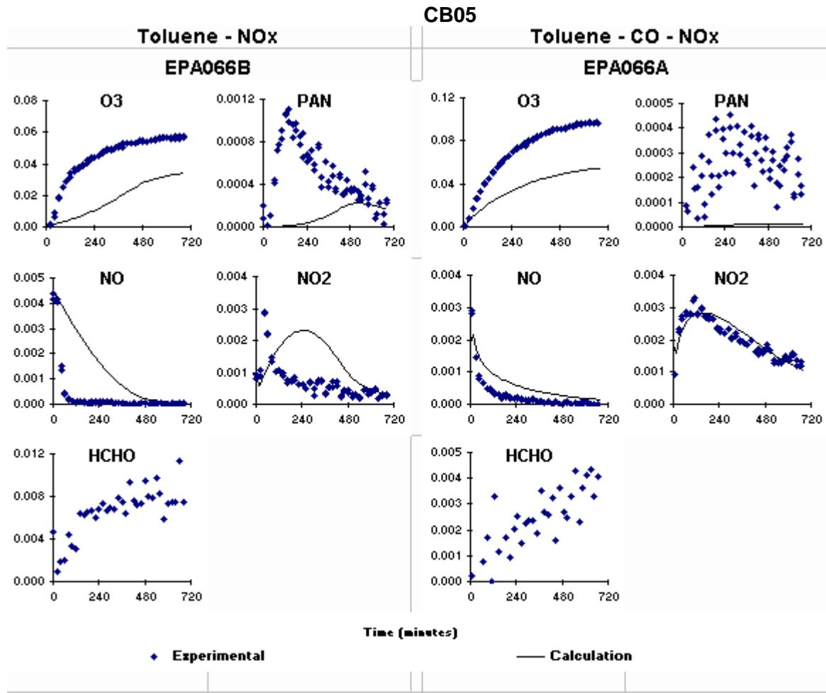
**Figure 4-13.** CB05 simulation of two toluene experiments in the EPA chamber at UCR.
