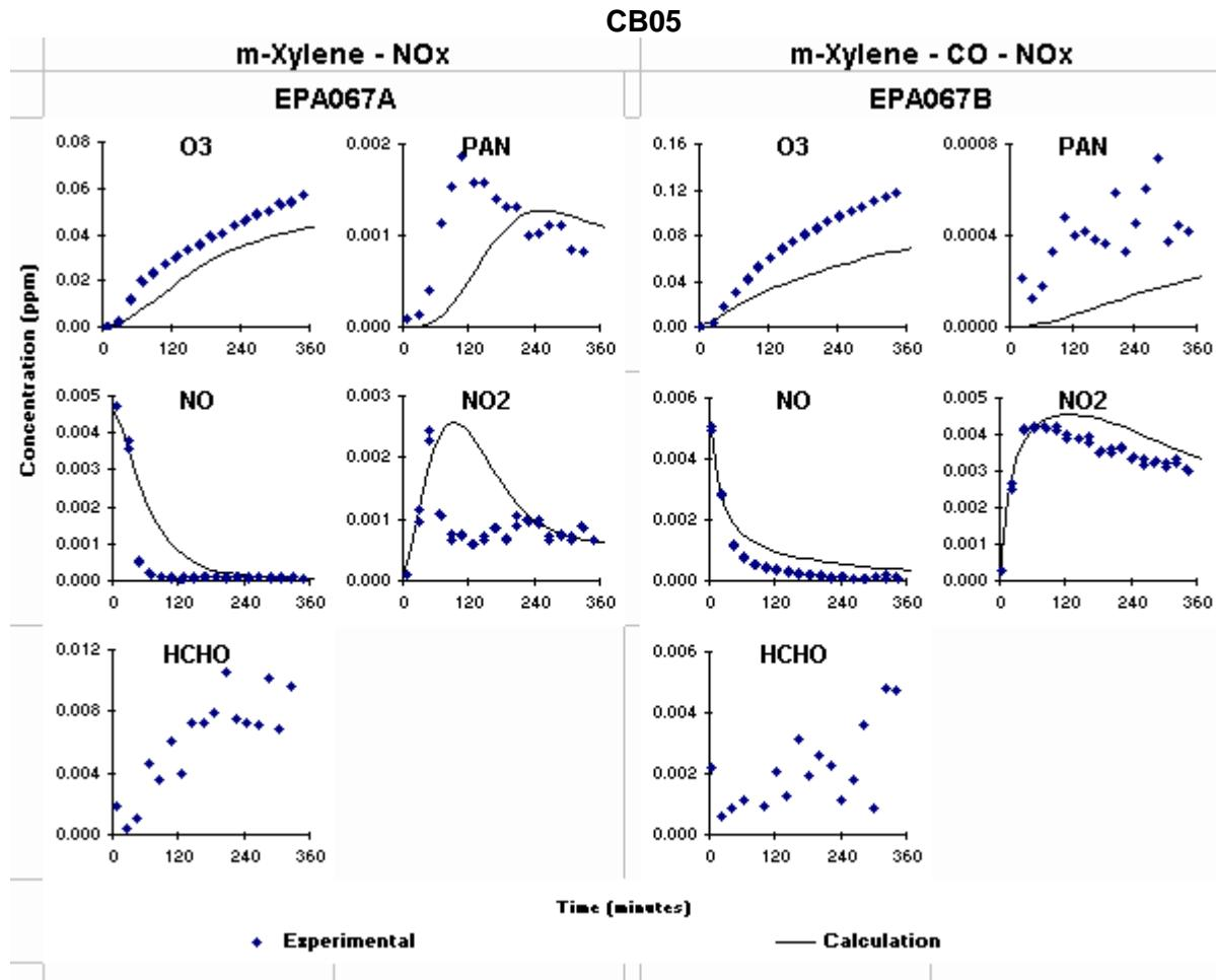
**Figure 4-15.** CB05 simulation of two xylene experiments in the EPA chamber at UCR.
