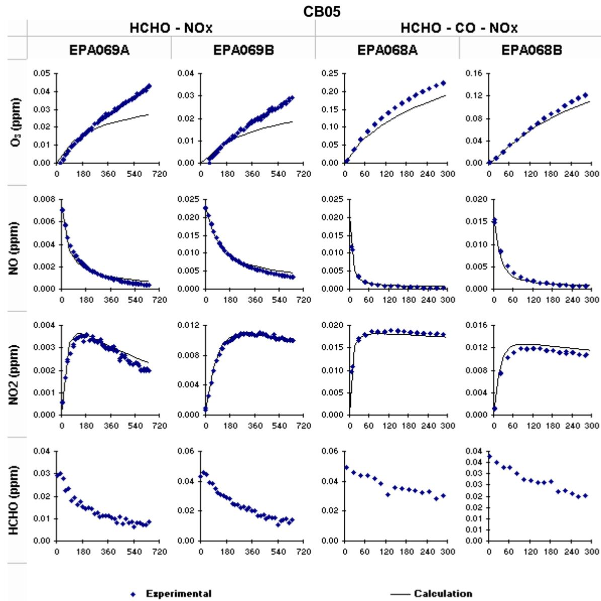
**Figure 4-8.** CB05 simulation of four formaldehyde experiments in the EPA chamber at UCR.
