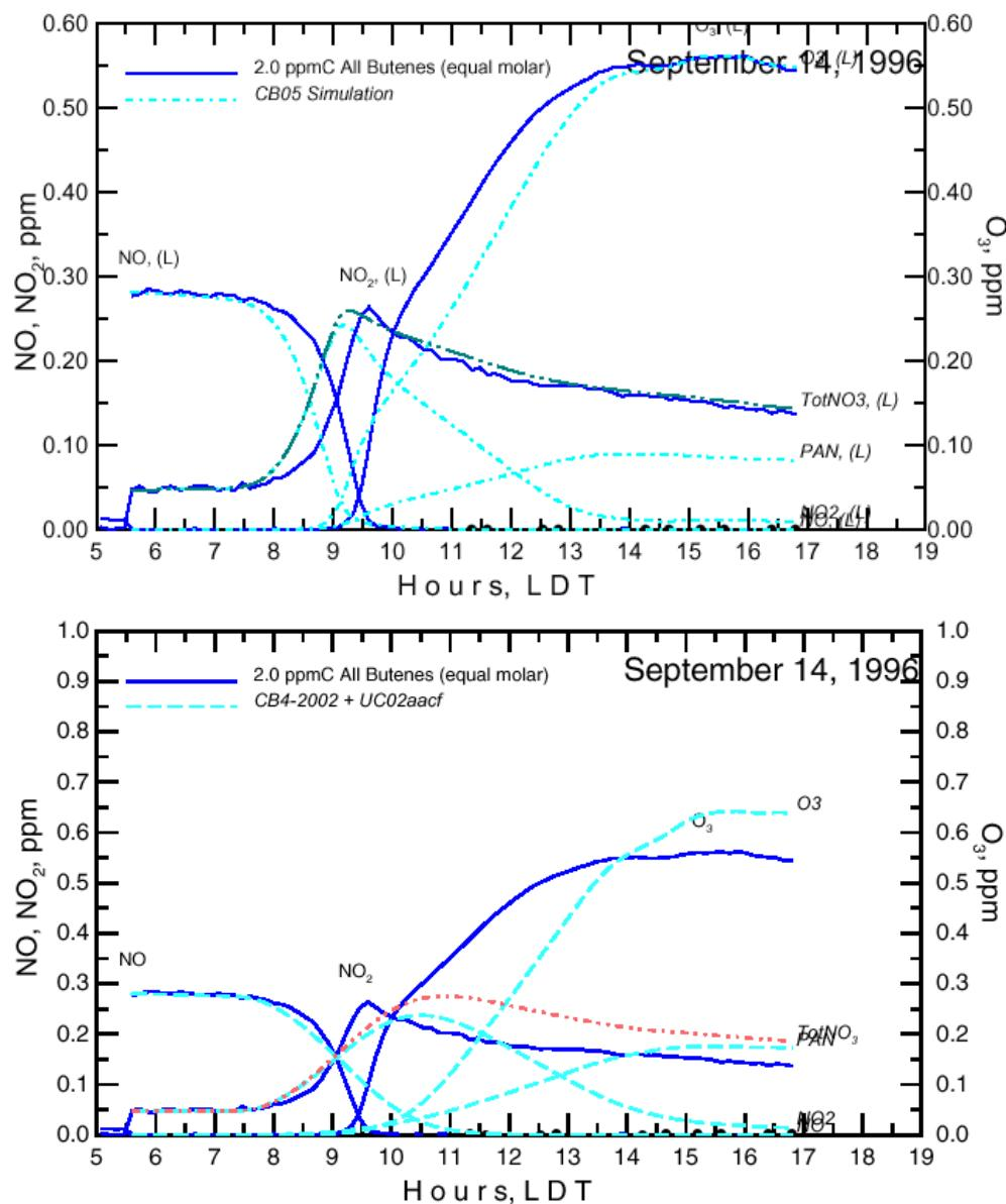
**Figure 4-5.** Comparison of CB05 (top) and CB4-2002 (bottom) simulations of UNC experiment September 14, 1996 (blue chamber) with an equimolar mixture of all butenes (1-butene, cis-2-butene, trans-2-butene, isobutene).
