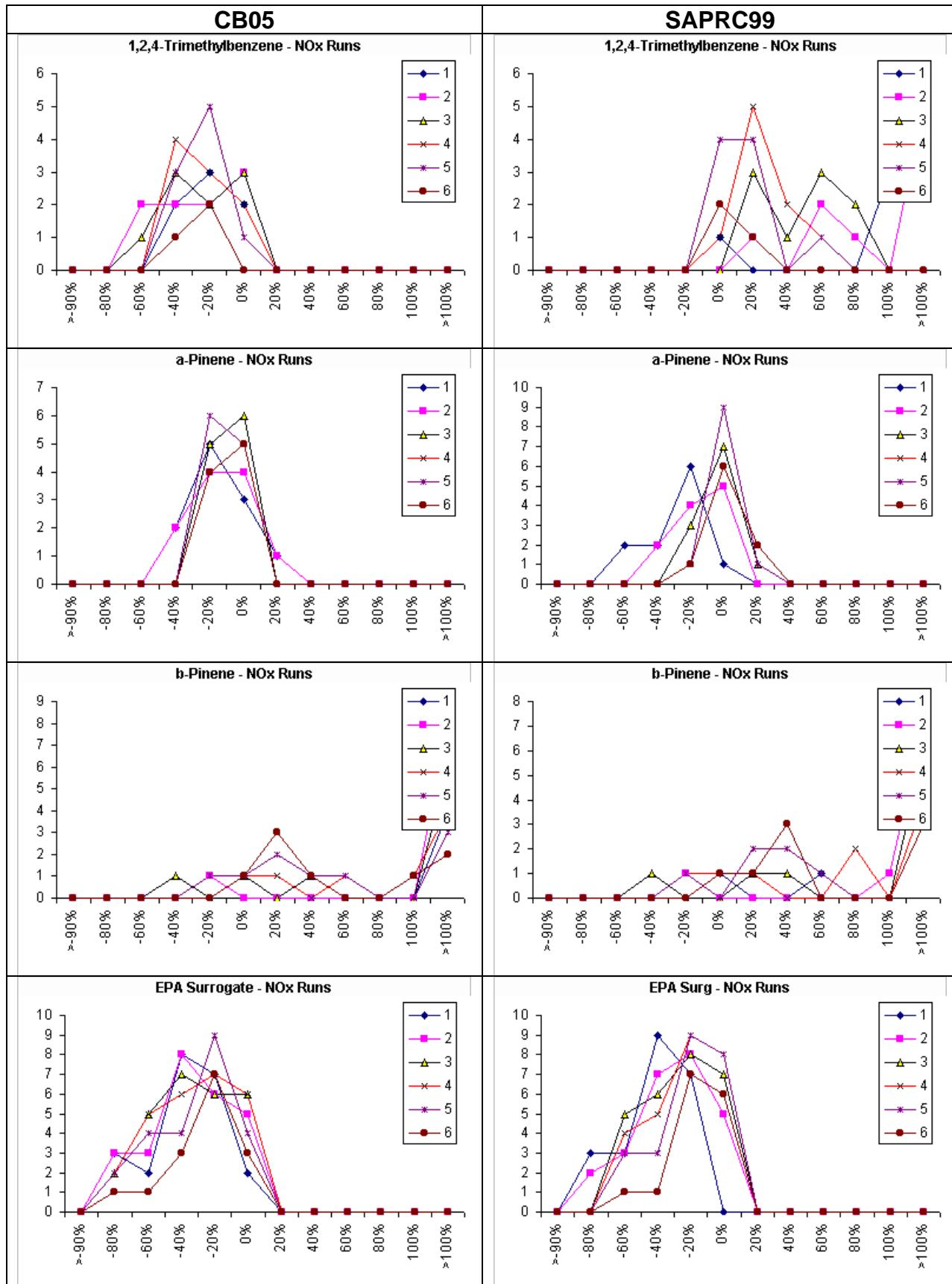
**Figure 4-16.** (continued). Bias in oxidant production (O<sub>3</sub>-NO) at hours 1-6 in UCR chamber experiments for the CB05 and SAPRC99 mechanisms, by compound.
