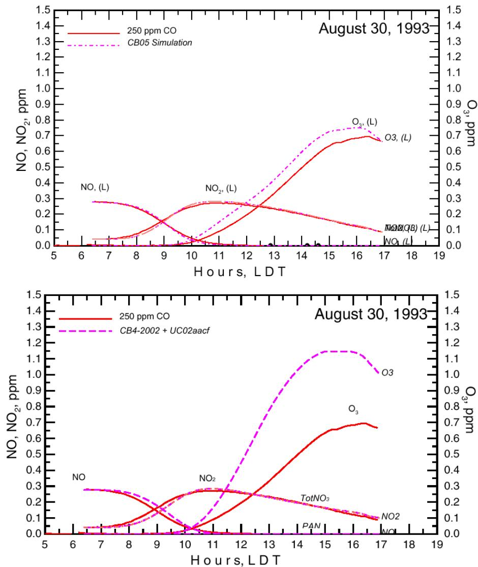
**Figure 4-1.** Comparison of CB05 (top) and CB4-2002 (bottom) simulations of UNC carbon monoxide experiment August 30, 1993 (red).
