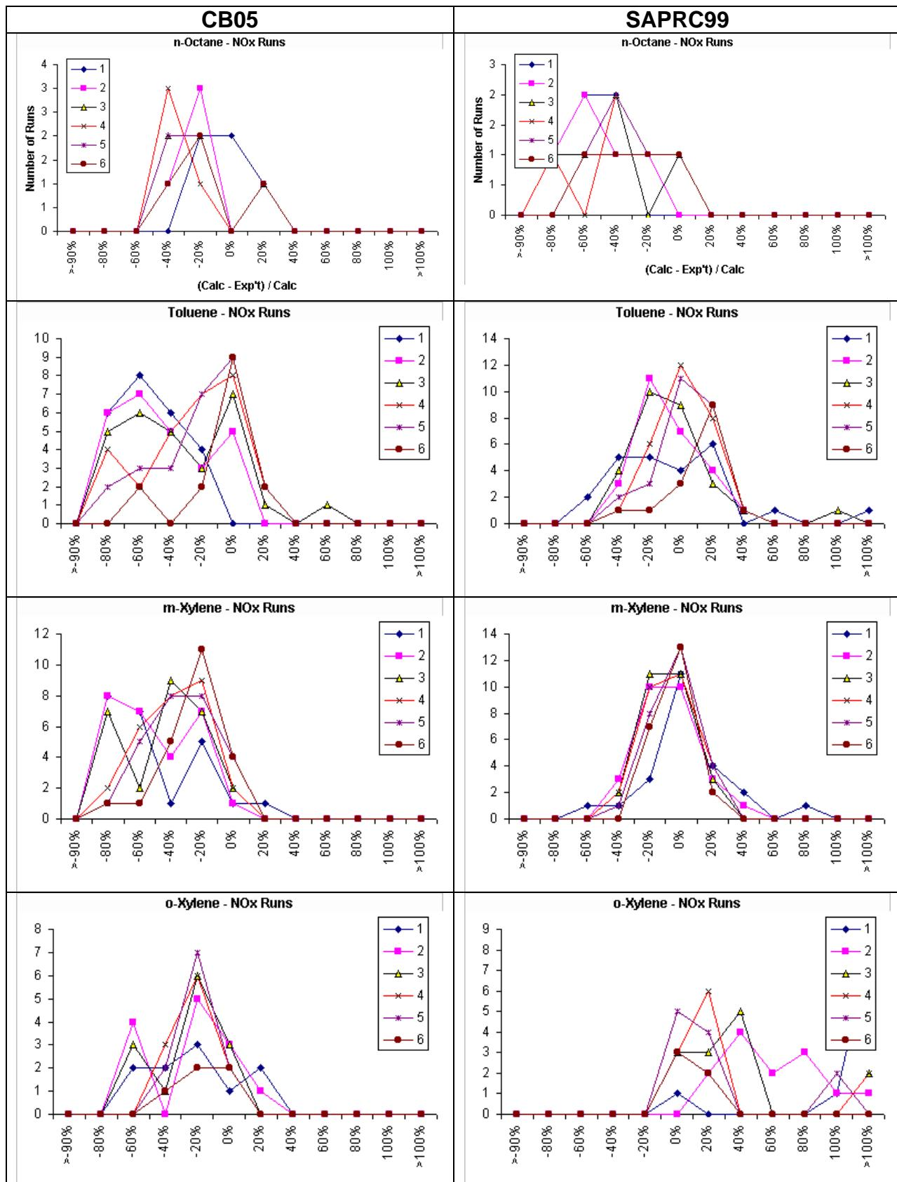
**Figure 4-16.** (continued). Bias in oxidant production ( $O_3$ -NO) at hours 1-6 in UCR chamber experiments for the CB05 and SAPRC99 mechanisms, by compound.
