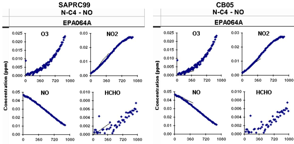
**Figure 4-11.** SAPRC99 (left) and CB05 (right) simulation of a butane experiment in the EPA chamber at UCR.
